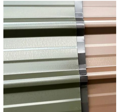
Figure 1. Pressure marring is visible these sections of formed COLORSTEEL® as a glossy wash pattern.
